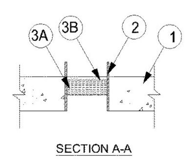
1. **Floor or Wall Assembly** — Min 4-1/2 in. (114 mm) thick reinforced lightweight or normal weight (100-150 pcf or 1600-24009 kg/m<sup>3</sup>) concrete. Wall may also be constructed of any UL Classified **Concrete Blocks\***. Max diam of opening is 6 in. (152 mm)
