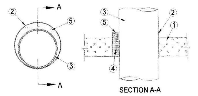
1. Floor or Wall Assembly — Min 4-1/2 in. thick reinforced lightweight or normal weight (100-150 pcf) concrete. Wall may also be constructed of any UL Classified Concrete Blocks\*.
