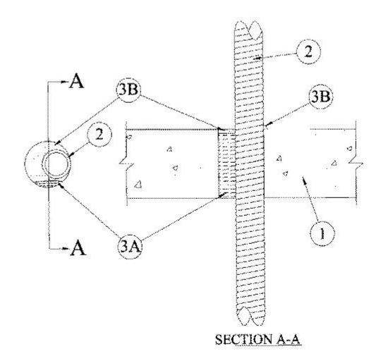
1. **Floor or Wall Assembly** — Min 4-1/2 in.(114 mm) thick reinforced lightweight or normal weight (100-150 pcf) (1600-2400 kg/m<sup>3</sup>) concrete. Wall may also be constructed of any UL Classified **Concrete Blocks\*.** Max diam of opening is 3 in.(76 mm)
