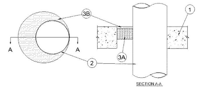
1. Floor or Wall Assembly — Min 4-1/2 in. (114 mm) thick reinforced lightweight or normal weight (100 - 150 pcf or 1600-2400 kg/m3) concrete. Floor may also be constructed of any min 6 in. (152 mm) thick hollow-core **Precast Concrete Units**\*. Wall may also be constructed of any UL Classified **Concrete Blocks**\*. Max diam of opening is 11-1/4 in. (286 mm). In hollow-core floors, max diam of opening is 7 in. (178 mm).
