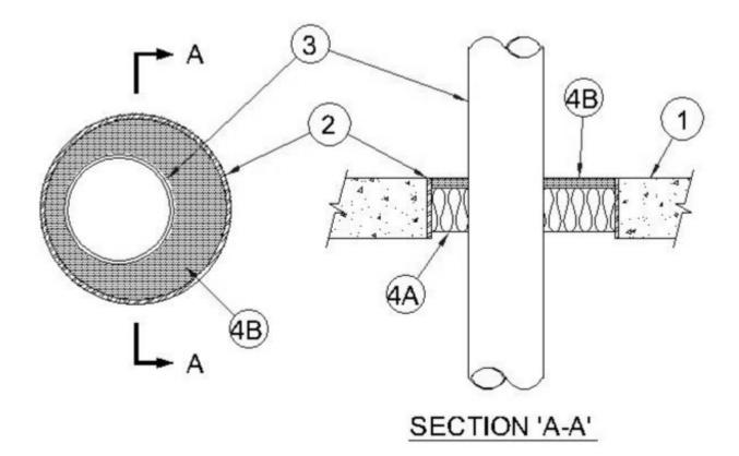
1. Floor or Wall Assembly — Min 4-1/2 in. (114 mm) thick reinforced lightweight or normal weight (100-150 pcf or 1600-2400 kg/m³) concrete. Floor may also be constructed of any min 6 in. thick UL Classified hollow-core Precast Concrete Units\*. Wall may also be constructed of any UL Classified Concrete Blocks\*. Max diam of opening is 6 in. (152 mm)
