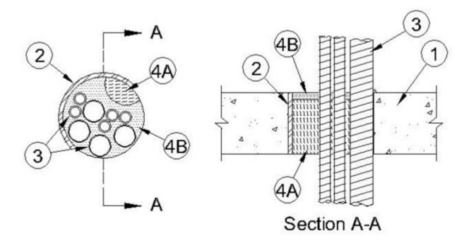
1. Floor or Wall Assembly — Min 4-1/2 in. (114 mm) thick reinforced lightweight or normal weight (100-150 pcf or 1600-2400 kg/m³) concrete. Floor assembly may also be constructed of any min 6 in. (152 mm) thick UL Classified hollow-core **Precast Concrete Units\***. Wall may also be constructed of any UL Classified **Concrete Blocks\***. Max diam of opening is 6 in. (152 mm).
