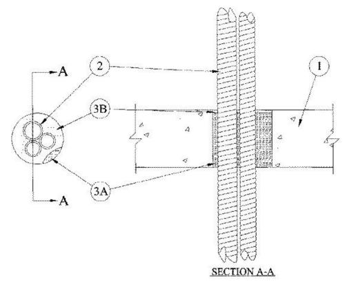
1. Floor or Wall Assembly — Min 4-1/2 in. (114 mm) thick reinforced lightweight or normal weight (100-150 pcf or 1600-2400 kg/m³) concrete. Wall may also be constructed of any UL Classified Concrete Blocks\*. Max diam of opening is 4 in. (102 mm).
