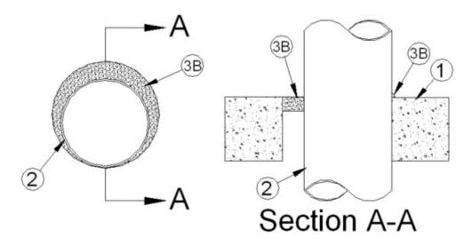
1. Floor or Wall Assembly — Min 4-1/2 in. (114 mm) thick reinforced lightweight or normal weight (100-150 pcf or 1600-2400 kg/m<sup>3</sup>) concrete. Floor may also be constructed of any min 6 in. (152 mm) thick UL Classified hollow-core **Precast Concrete Units\***. Wall may also be constructed of any UL Classified **Concrete Blocks\***. Max diam of opening is 14 in. (356 mm).
