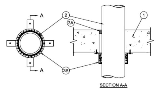
1. **Floor or Wall Assembly** — Min 4-1/2 in. (114 mm)thick reinforced lightweight or normal weight (100-150 pcf 1600-2400 kg/m<sup>3</sup>) concrete. Wall may also be constructed of any UL Classified **Concrete Blocks**\*. Floor may also be constructed of any min 6 in. (152 mm) thick UL Classified hollow-core **Precast Concrete Units**\*. Max diam of opening is 5 in. (127 mm)
