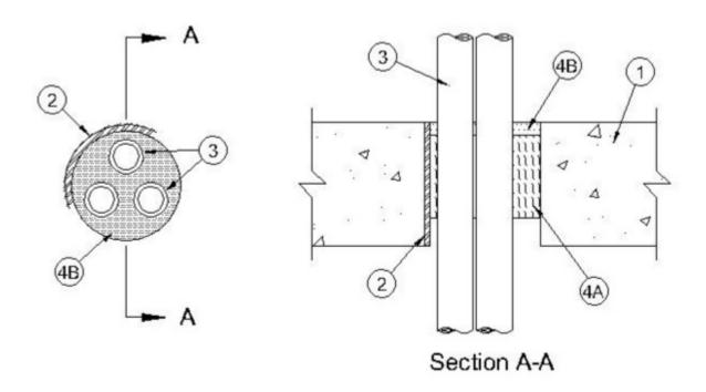
1. Floor or Wall Assembly — Min 4-1/2 in. (114 mm) thick reinforced lightweight or normal weight (100-150 pcf or 1600-2400 kg/m<sup>3</sup>) concrete floor. Floor may also be constructed of any min 6 in. (152 mm) thick hollow-core **Precast Concrete Units\***. Wall may also be constructed of any UL Classified **Concrete Blocks\***. Max diam of opening is 6 in. (152 mm).
