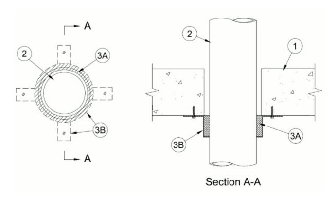
1. **Floor or Wall Assembly** — Min 4-1/2 in. (114 mm) thick reinforced lightweight or normal weight (100-150 pcf or 1600-2400 kg/m<sup>3</sup>) concrete. Wall may also be constructed of any UL Classified **Concrete Blocks\***. Floor may also be constructed of any min 6 in. (152 mm) thick UL Classified hollow-core **Precast Concrete Units\***. Opening to be max 1-1/16 in. (27 mm) larger than outside diam of nonmetallic pipe. Max diam of opening is 6 in. (152 mm).
