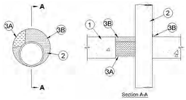
1. **Floor or Wall Assembly** — Min 4-1/2 in. (114 mm) thick reinforced lightweight or normal weight (100-150 pcf or 1600-2400 kg/m<sup>3</sup>) concrete. Wall may also be constructed of any UL Classified **Concrete Blocks\***. Max diam of opening is 4 in. (102 mm).
