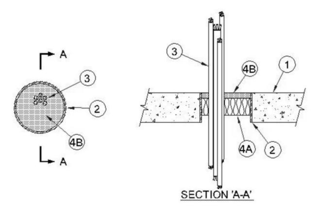
1. Floor or Wall Assembly — Min 4-1/2 in. (114 mm) thick reinforced lightweight or normal weight (100-150 pcf or 1600-2400 kg/m<sup>3</sup>) concrete. Floor may also be constructed of any min 6 in. thick UL Classified hollow-core **Precast Concrete Units\***. Wall may also be constructed of any UL Classified **Concrete Blocks\***. Max diam of opening is 6 in. (152 mm).
