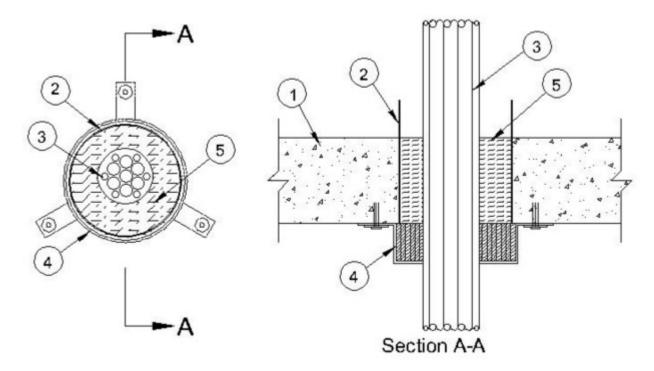
1. Floor or Wall Assembly — Min 4-1/2 in. (114 mm) thick lightweight or normal weight (100-150 pcf or 1600-2400 kg/m<sup>3</sup>) concrete floor. Wall may also be constructed of any UL Classified **Concrete Blocks\***. Floor may also be constructed of any min 6 in. (152 mm) thick hollow core UL Classified **Precast Concrete Units\***. Max diam opening is 6 in (150 mm).
