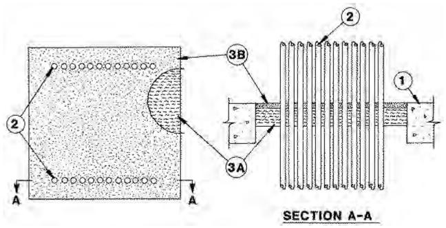
1. **Floor Or Wall Assembly** — Min 4-1/2 in. (114 mm) thick reinforced normal weight (145-150 pcf (2320-2400 kg/cu meter)) concrete. Wall may also be constructed of any UL Classified **Concrete Blocks\*.** Max area of opening is 289 sq in. (1860 sq cm) with max dimension of 17 in. (432 mm).
