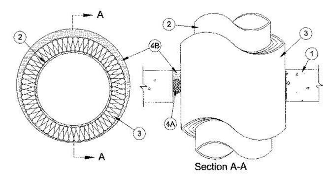
1. **Floor or Wall Assembly** — Min 4-1/2 in. (114 mm) thick reinforced lightweight or normal weight (100-150 pcf or 1600-2400 kg/m<sup>3</sup>) concrete. Wall may also be constructed of any UL Classified **Concrete Blocks**\*. Floor may also be constructed of any 6 in. (152 mm) thick UL Classified hollow-core **Precast Concrete Units**\*. Max diam of opening is 16 in. (406 mm) When precast concrete units are use, max diam of opening is 7 in. (178 mm)
