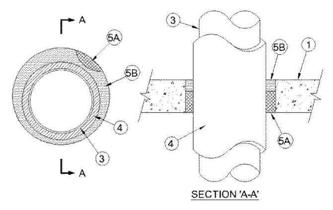
1. **Floor or Wall Assembly** — Min 2-1/2 in. (64 mm) thick reinforced light weight or normal weight (100-150 pcf or 1600-2400 kg/m<sup>3</sup>) concrete. Wall may also be constructed of any UL Classified **Concrete Blocks\***. Max diam of opening is 8-1/2 in.
