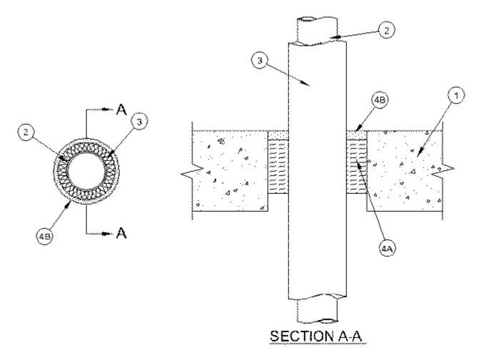
1. **Floor or Wall Assembly** — Min 4-1/2 in. thick reinforced lightweight or normal weight (100-150 pcf) concrete. Wall may also be constructed of any UL Classified **Concrete Blocks**\*. Max diam of opening is 8 in.
