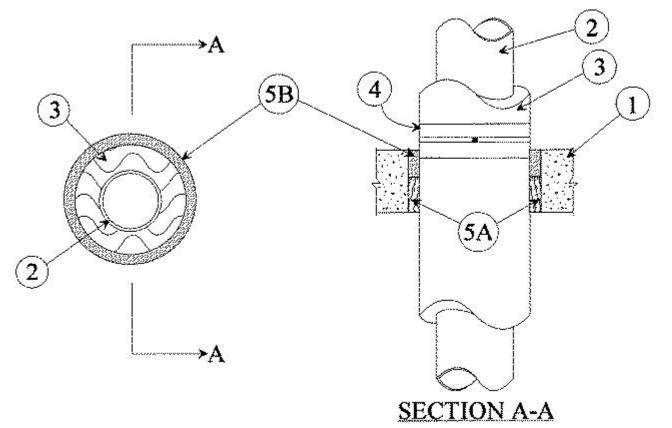
1. Floor or Wall Assembly — Min 4-1/2 in. (114 mm) thick reinforced lightweight or normal weight (100-150 pcf) (1600-2400 kg/m<sup>3</sup>) concrete floor or min 6-1/2 in. (165 mm) thick reinforced lightweight or normal weight concrete wall. Wall may also be constructed of any UL Classified **Concrete Blocks\*.** Max diam of opening is 18 in. (457 mm)
