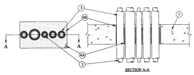
1. **Floor or Wall Assembly** — Min 5-1/2 in. (140 mm) thick reinforced lightweight or normal weight (100-150 pcf) (1600-2400 kg/m³) concrete. Wall may also be constructed of any UL Classified **Concrete Blocks\***. Max area of opening is 128 sq in. (3251 mm) with max dimension of 16 in.
