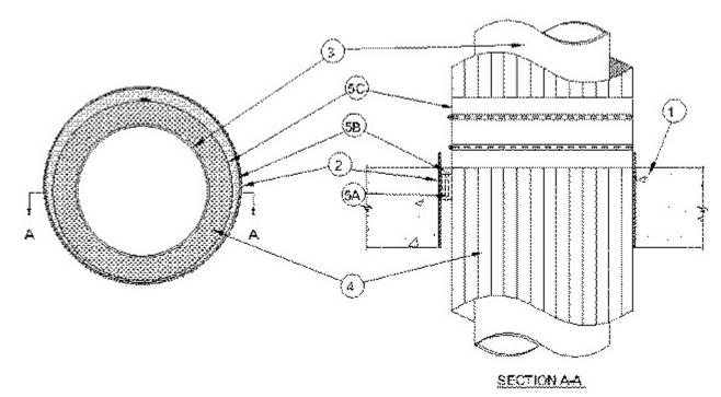
1. **Floor or Wall Assembly** — Min 4-1/2 in. (114 mm) thick reinforced lightweight or normal weight (100-150 pcf) (1600-2400 kg/m³) concrete. Floor assembly may also be constructed of any min 6 in. (152 mm) thick UL Classified hollow-core **Precast Concrete Units\***. Wall may also be constructed of any UL Classified **Concrete Blocks\***. Max diam of opening 28 in. (711 mm) Max diam of opening in floors constructed of hollow-core concrete is 7 in. (178 mm)
