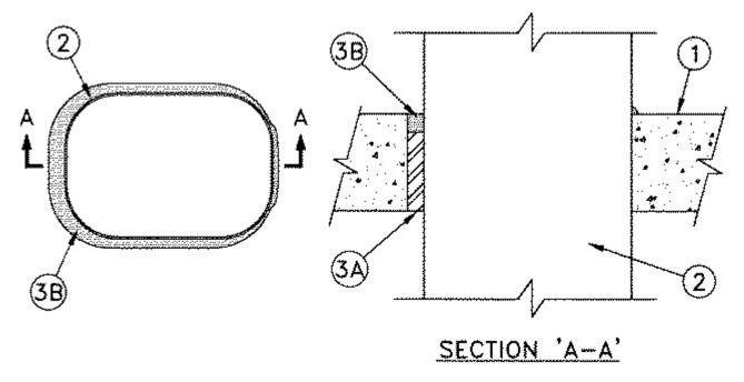
1. **Floor or Wall Assembly** — Min 4-1/2 in. (114 mm) thick reinforced light weight or normal weight (100-150 pcf or 1600-2400 kg/m<sup>3</sup>) concrete floor or min 5 in. (127 mm) thick light weight or normal weight concrete wall. Wall may also be constructed of any UL Classified **Concrete Blocks**\*. Max area of opening is 715 sq in. (4613 cm<sup>2</sup>) with max dimension of 37-1/4 in. (946 mm).
