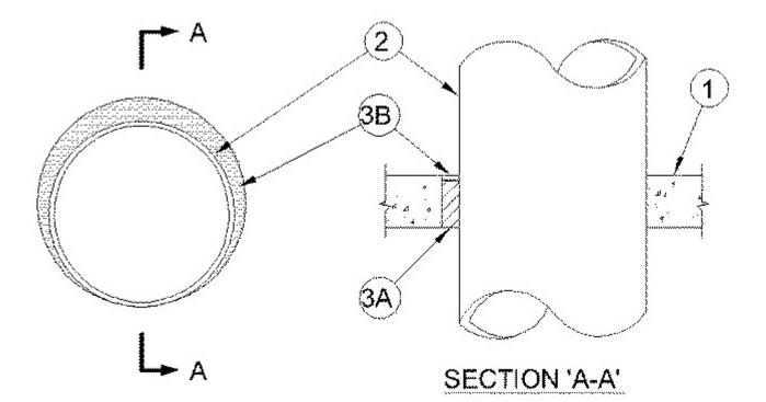
1. **Floor or Wall Assembly** — Min 4-1/2 in. (114 mm) thick floor or 5 in. (127 mm) thick wall of reinforced lightweight or normal weight (100-150 pcf or 1600-2400 kg/m<sup>3</sup>) concrete. Wall may also be constructed of any UL Classified **Concrete Blocks**\*. Max diam of opening is 28 in. (711 mm).
