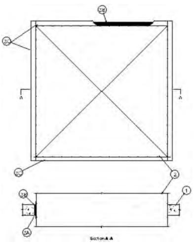
1. **Floor or Wall Assembly** — Min 6 in. (152 mm) thick reinforced lightweight or normal weight (100-150 pcf or 1600-2400 kg/m<sup>3</sup>) concrete. Wall may also be constructed of any UL Classified **Concrete Blocks\***. Max size of opening is 73.7 sq ft (6.8 m<sup>2</sup>) with a max width of 104 in. (264 cm).
