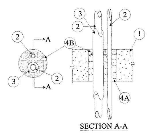
1. **Floor or Wall Assembly** — Min 4-1/2 in. (114 mm) thick reinforced lightweight or normal weight (100-150 pcf) (1600-2400 kg/m<sup>3</sup>) concrete floor or min 5-1/4 in. (133 mm) thick reinforced lightweight or normal weight concrete wall. Wall may also be constructed of any UL Classified **Concrete Blocks\***. Floor may also be constructed of any min 6 in. (152 mm) thick UL Classified hollow-core **Precast Concrete Units\***. Max diam of opening is 4 in. (102 mm).
