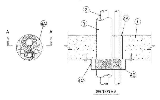
1. **Floor or Wall Assembly** — Min 4-1/2 in. (114 mm) thick reinforced lightweight or normal weight (100-150 pcf or 1600-2400 kg/m<sup>3</sup>) concrete. Wall may also be constructed of any UL Classified **Concrete Blocks**\*. Max diam of opening 6 in.
