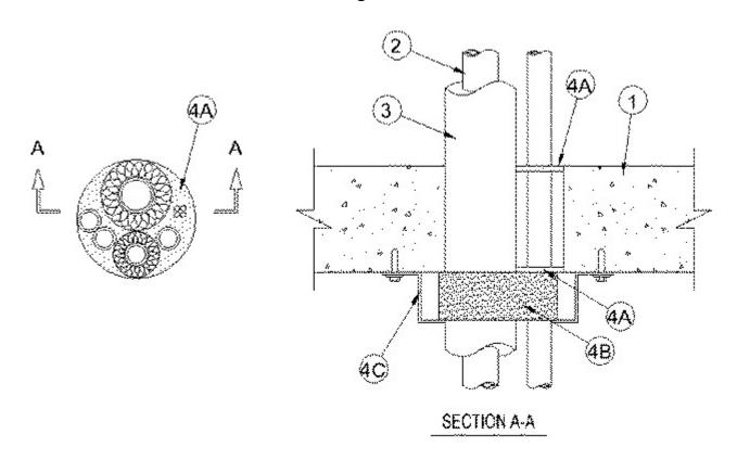
1. **Floor or Wall Assembly** — Min 2-1/2 in. (64 mm) thick reinforced lightweight or normal weight (100-150 pcf or 1600-2400 kg/m<sup>3</sup>) concrete. Wall may also be constructed of any UL Classified **Concrete Blocks**\*. Max diam of opening 5 in. (127 mm).
