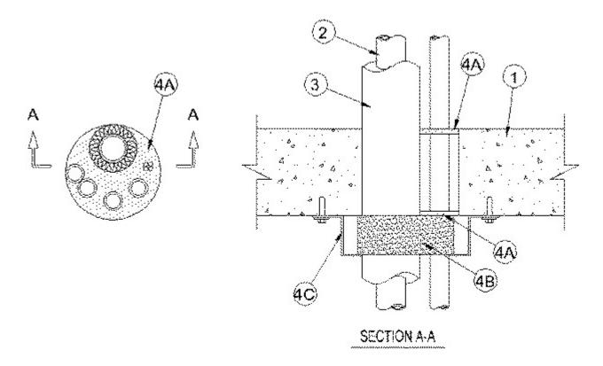
1. **Floor or Wall Assembly** — Min 2-1/2 in. (64 mm) thick reinforced lightweight or normal weight (100-150 pcf or 1600-2400 kg/m<sup>3</sup>) concrete. Wall may also be constructed of any UL Classified **Concrete Blocks\***. Max diam of opening 5 in. (127 mm)
