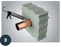
Apply caulking as required to close remaining gap to both sides of wall assembly; providing a fire smoke and gas resistant seal. Spread caulking smoothly and evenly all around.
