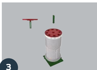
3 Re-install cap & insert whiskers
