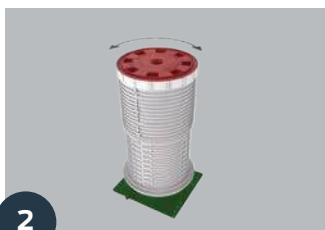
2 Lock outer sleeve in place
