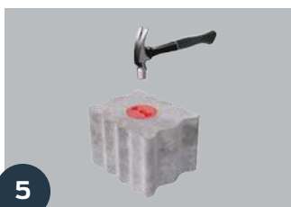
Knock out safety cap with hammer or screwdriver
