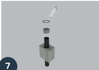
3 Re-install cap & insert whiskers
