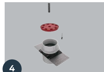
4 Re-install cap & insert whiskers
