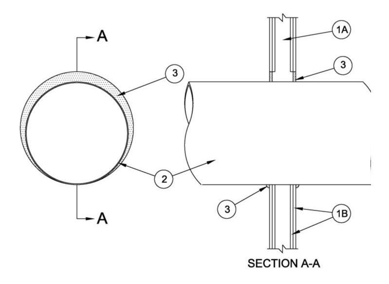
1. **Wall Assembly** — The 1 or 2 hr fire-rated gypsum board/stud wall assembly shall be constructed of the materials and in the manner described in the individual U300, U400, V400 or W400 Series Wall and Partition Design in the UL Fire Resistance Directory and shall include the following construction features:
