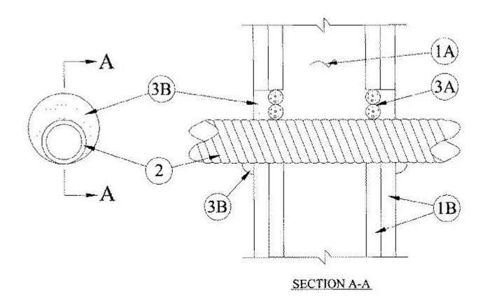
1. **Wall Assembly** — The 1 or 2 hr fire-rated gypsum wallboard/stud wall assembly shall be constructed of the materials and in the manner specified in the individual U300 or U400 Series Wall and Partition Designs in the UL Fire Resistance Directory and shall include the following construction features:
