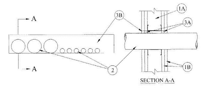
1. **Wall Assembly** — The 1 or 2 hr fire-rated gypsum board/stud wall assembly shall be constructed of the materials and in the manner described in the individual U300, U400 or V400 Series Wall and Partition Design in the UL Fire Resistance Directory and shall include the following construction features:
