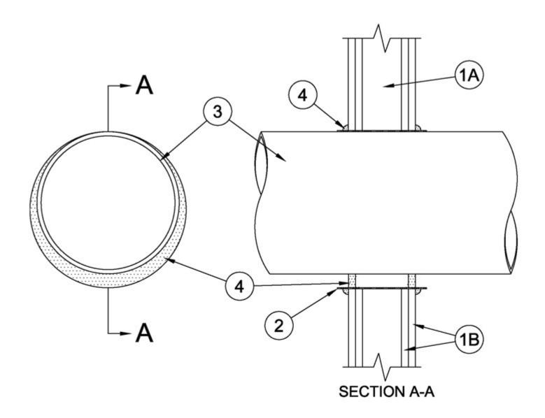
1. **Wall Assembly** — The 1 or 2 hr fire rated gypsum board/stud wall assembly shall be constructed of the materials and in the manner specified in the individual U300, U400, V400 or W400 Series Wall and Partition Designs in the UL Fire Resistance Directory and shall include the following construction features:
