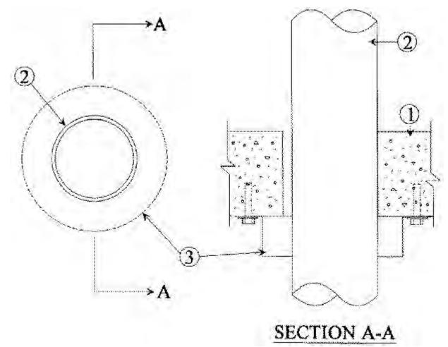
1. **Floor or Wall Assembly** — Min 4-1/2 in. thick reinforced lightweight or normal weight (100-150 pcf) concrete. Wall may also be constructed of any UL Classified **Concrete Blocks\*.** Floor may also be constructed of any min 6 in. thick UL Classified hollow-core **Precast Concrete Units\*.** Max diam of opening is 7 in.
