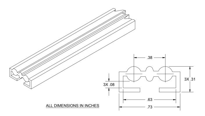
Engineered sound insulation lining, minimizes the occurrence of frictional noises caused by thermal expansion of the pipes and protects against contact between dissimilar materials. Attaches to ends of HOLDRITE Stout Brackets™ or around pipes to provide isolation from structure. Also provide sound isolation between metal loop hangers and piping. Available in 50' rolls.
