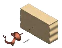
LOOSEN UPPER CLAMP AND SECURE TO FRAMING. (FIG. 1)
