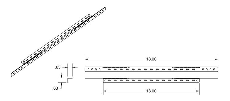
A versatile, Copper-Bonded<sup>™</sup> bracket providing a platform for horizontal or vertical tube support. Also ideal for shower head, diverter and tub spout applications. Copper-Bonded<sup>™</sup> feature allows tubes to be soldered directly to bracket. Heat the pipe, not the bracket.
