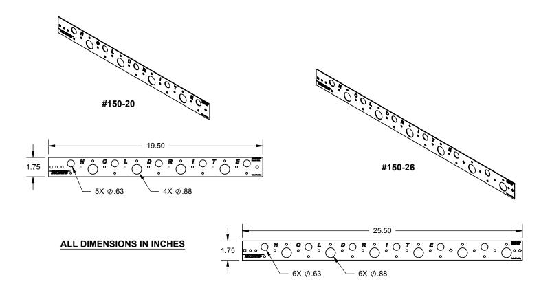
The HOLDRITE® #150-20 and #150-26 are Copper-Bonded™ steel brackets for support of 1/2" and 3/4" pipes on 4" or 8" centers. The #150-20 & #150-26 position copper water supplies for sinks, water closets, and other fixtures. When soldering, heat the pipe, not the bracket.
