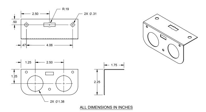
The HOLDRITE® #121-DS is a 20 gage galvanized steel bracket the supports dual lines of 1/2", 3/4" or 1" Copper, PEX or CPVC tubing at 1-1/4" center line height. The hole pattern on the 90 $^\circ$  base allows for attachment to any flat surface. The bracket can also be suspended by 3/8" threaded rod.
