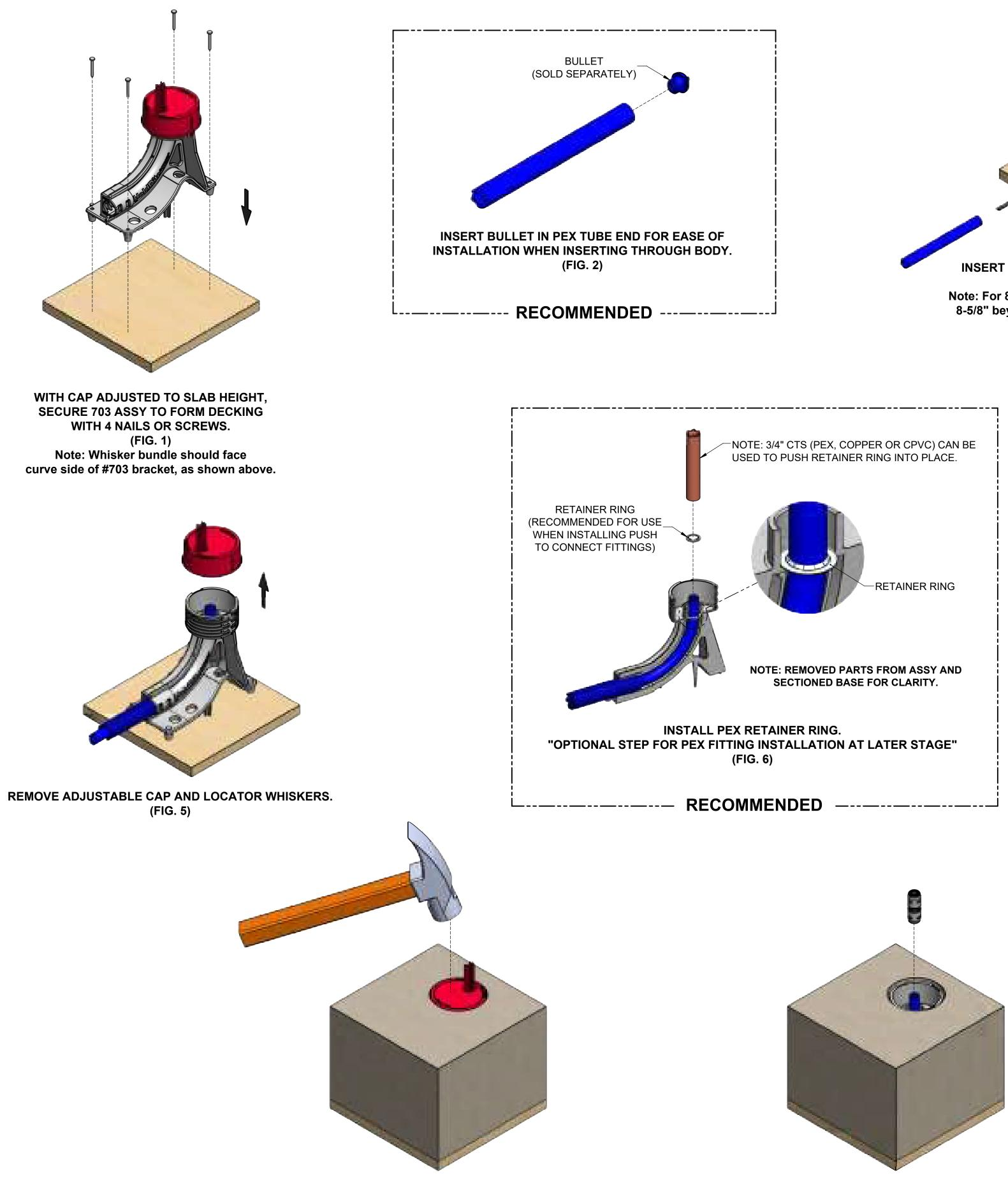
WHEN IT IS TIME TO CONNECT TO PEX TUBING, REMOVE ADJUSTABLE CAP AND LOCATOR WHISKERS USING HAMMER. (FIG. 9)
