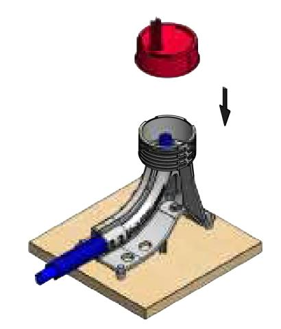
REATTACH ADJUSTABLE CAP AND LOCATOR WHISKERS AND SET TO REQUIRED SLAB HEIGHT. (FIG. 7)
