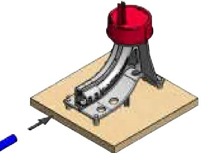
INSERT 1/2" PEX TUBE THROUGH 703 BODY. (FIG. 3A) Note: For 8" slab height PEX tubing should extend 8-5/8" beyond corrugated sleeving, prior to PEX insertion into bracket.
