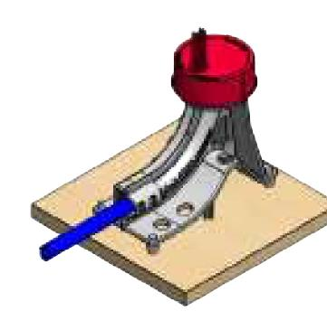
PUSH TUBE THROUGH UNTIL IT HITS BOTTOM SIDE OF CAP. (FIG. 3B)
