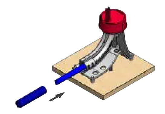
SLIDE PLASTIC CORRUGATED SLEEVING OVER PEX TUBE UNTIL LOCKED IN PLACE. (FIG. 4)
