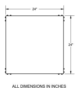
The QUICKSTAND™ #40-S-24- (A or U) stands safely elevates water heaters and other equipment above the floor (1,200 lbs rating).
