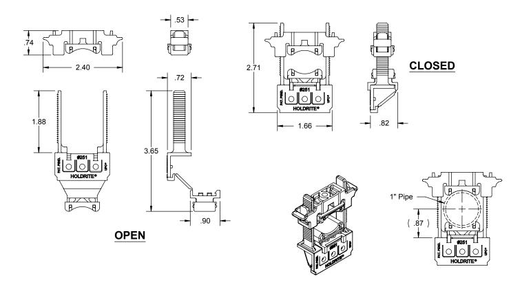
The HOLDRITE® Rapid Clamp™ #251 is a variable closure tube clamp designed to attach securely to the HOLDRITE #170 Bracket without the use of screws. Clamp supports up to 1"CTS tube size and is compatible with any tubing including Copper, PEX, CPVC tubing, and conduit. The #251 Rapid Clamp is UPC listed.
