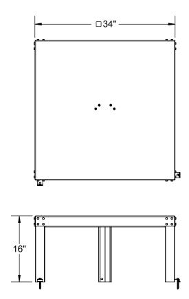
The QUICKSTAND™ #40-S-34-U stand safely elevates water heaters and other equipment above the floor (2,000 lbs rating).
